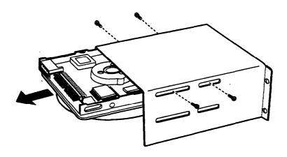
5. Replace the bracket inside the computer as shown below and secure it to the back panel with the four screws you removed earlier.
